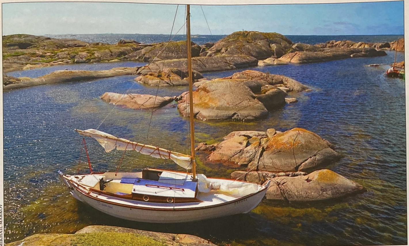
The 22'7" Kotik is a stretched version of Iain's Wee Seal design. The prototype was built in Holland and fitted out by owner Mikhail Markov in Finland. "The little draft of my boat is a huge advantage—we can always find good places to overnight, both in marinas and 'wild,'" says Markov. At least six more Kotiks have been built since Markov's WHITE FANG.
